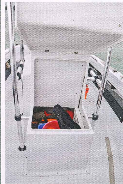
Above left: The forward seat lifts to expose stowage space in the front of the console. Above right: Switching, instruments and electronics are all flush mounted.
