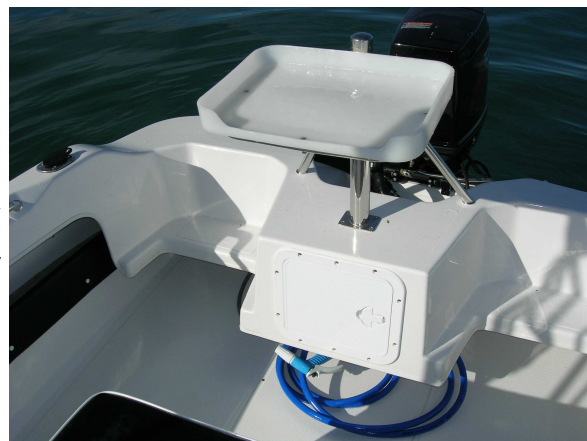
A bait board is mounted on the ski pole. The cutaways to either side can be fitted with squabs/
