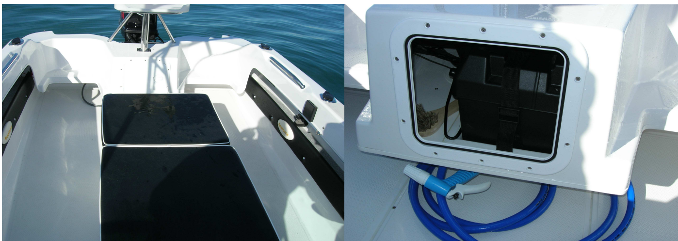
The battery is centrally placed in a protected transom locker The central storage bins double as seats and worktops.
