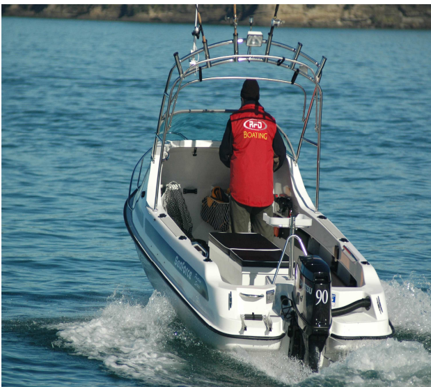
A heavy rubbing strip runs right around the hull.
